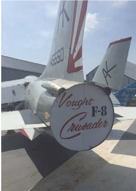
Visible exterior corrosion, sun damage, and worn-out surface paint on the tail of the F-8K Crusader before coming into the ARH in 2024. Photo credit: Intrepid Museum
