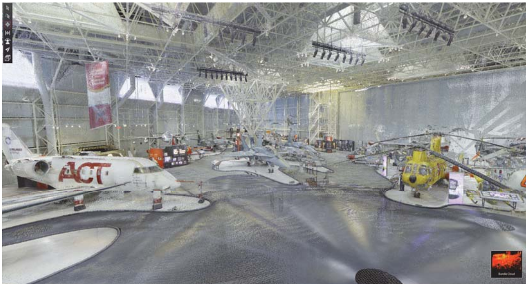
Point cloud data from LiDAR scanning the Canada Aviation and Space Museum floor
