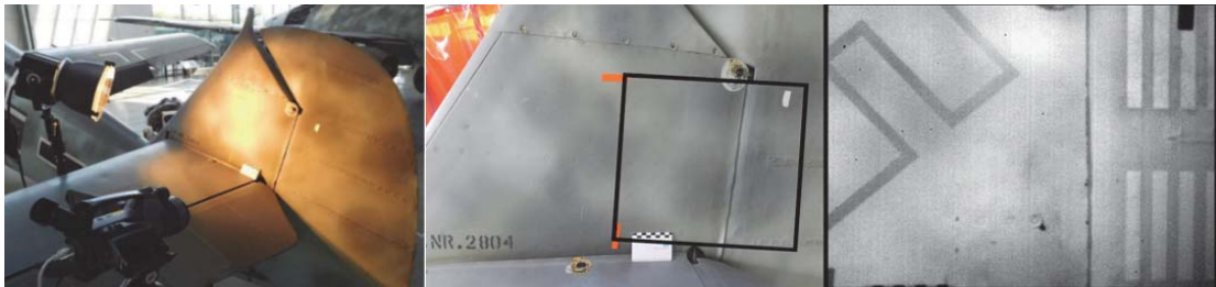
Left: Measurement setup for lock-in thermography with heat lamps and infrared camera on the tail of the Bf 109.
